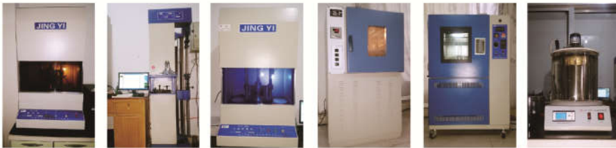
Vulkameter Electronic tensile Testing machine Mooney viscometer High temperature aging test chamber Ozone aging test chamber Aging test chamber
